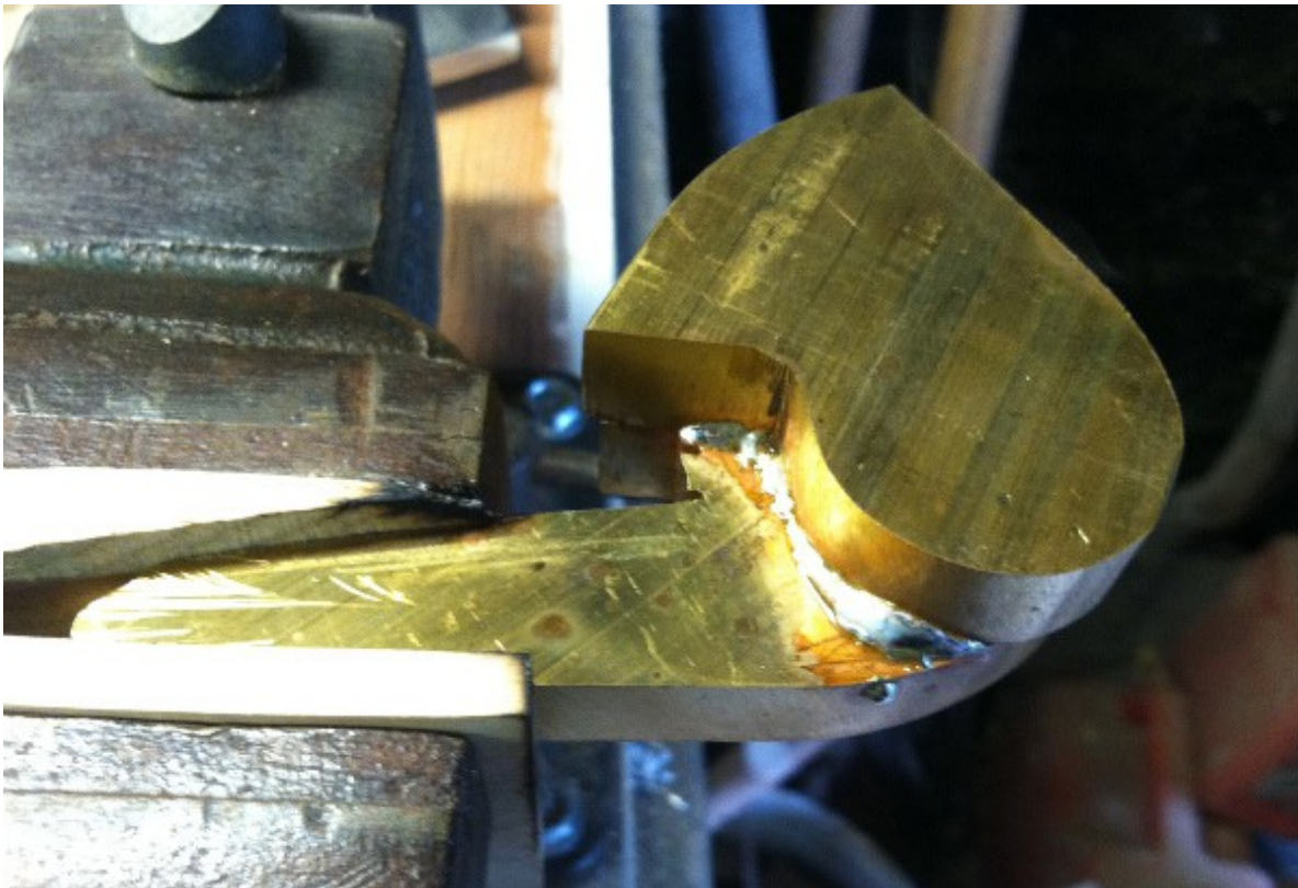
Figure E.2 Nut pieces soldered together for machining.
