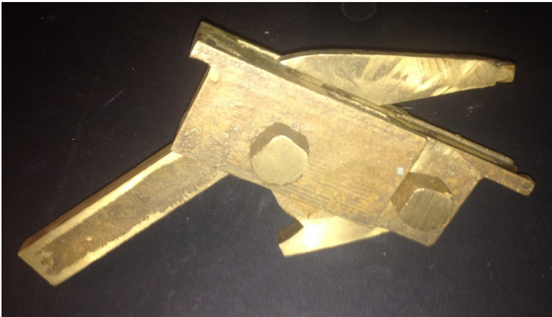
Figure C. Bronze cast trigger, modern reproduction, patterned after extant originals. Shown with the trigger tripped. (Thanks to Archos Arion for access.)
