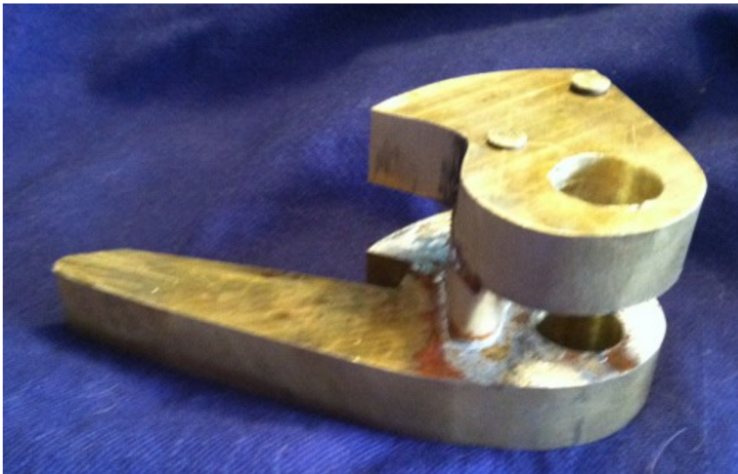
Figure E.4 Nut final assembly. The two parts have been split and the spreader and sear pivot installed and pinned.
