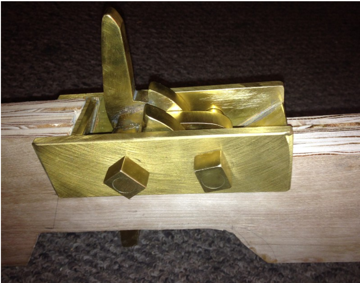
Figure I. Set into the 'roughed in' tiller body (Gen. 2). Ultimately, it will be pinned. This is a view that I would have liked to have had when trying to figure it out.
