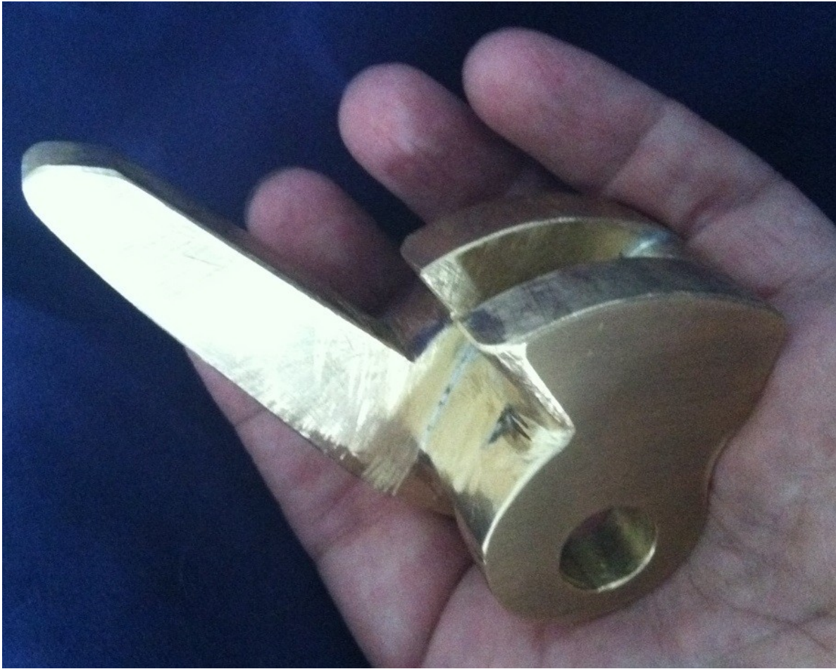
Figure E.5 Nut cleaned up and ready to install.
