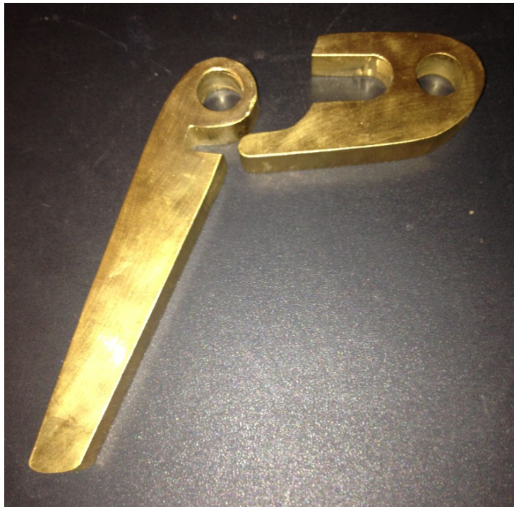
Figure G. The trigger lever and sear. This is the second set. The first set was cut thinner in order to fit the narrower cast bronze nut.
