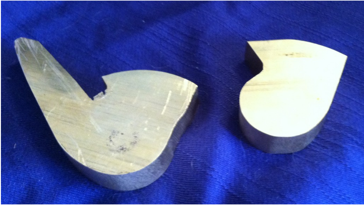
Figure E.1 Nut parts roughed out
